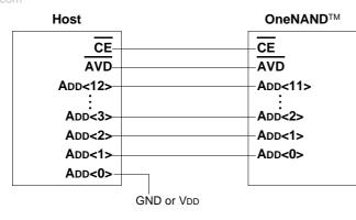
> If host uses byte-order typed address, ADD<0> can be used as byte/word selection pin.
