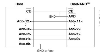
> If host uses byte-order typed address, ADD<0> can be used as byte/word selection pin.
