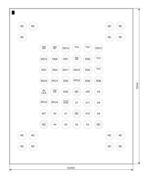
(TOP VIEW, Balls Facing Down) 63ball FBGA OneNAND<sup>™</sup> Chip 9.5mm x 12mm x max. 1.4mmt, Ball Pitch: 0.8mm
